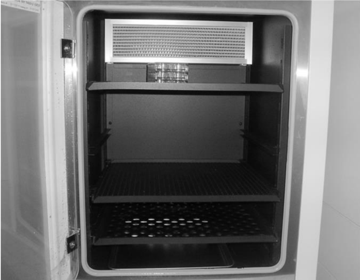
Figure 2: Far Infrared Ray CO 2 incubator (Yamashita, 2012)
