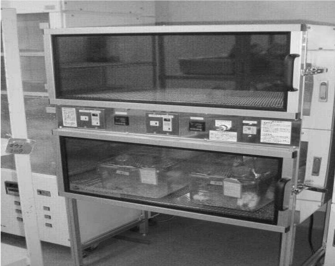
Figure 3: Far Infrared Ray animal raising apparatus (Yamashita, 2012)
