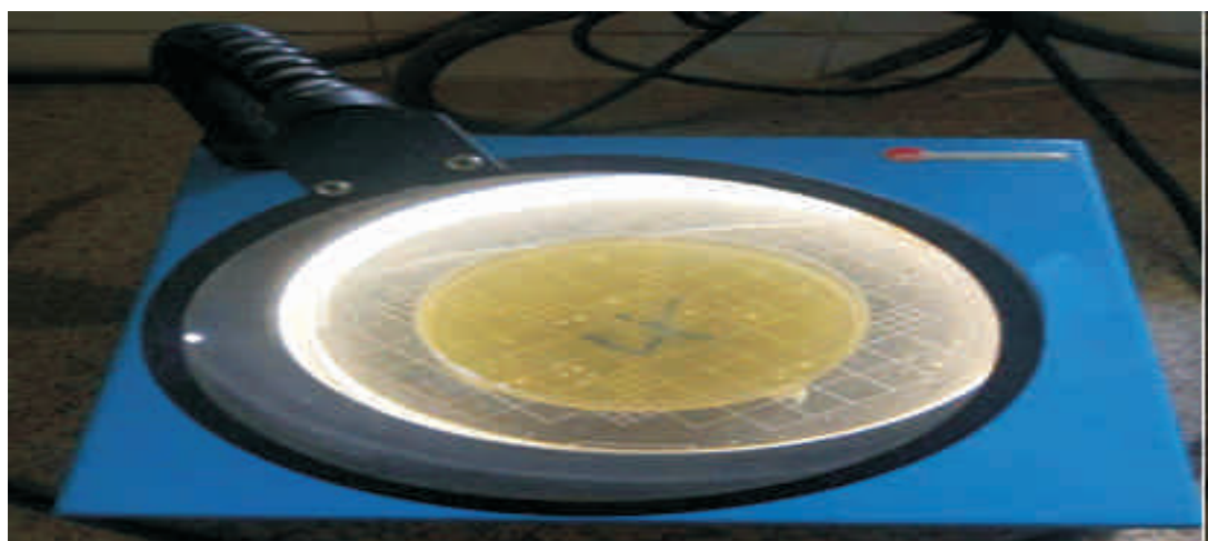
Plate 1: Colony count on nutrient agar Plate using colony counter
